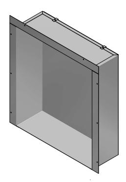
When building in , always keep a distance of minimum 10mm to the top ,sides,and back to avoid overheating
